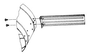
Figure 3 — Mounting Housing to Brackets
